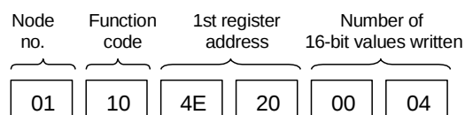
Figure 5 - ModBus Write Reply Message Example
